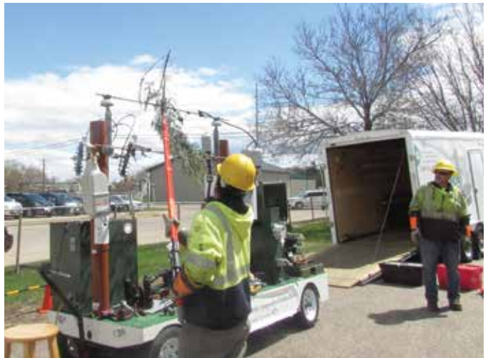
CWEC linemen, Jason Walter and Chris Tuszke, demonstrated to students in Wittenberg what happens when a tree branch comes in contact with an energized power line.
